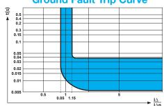
**UL 489**Branch Circuit Breaker with Ground Fault Relay
